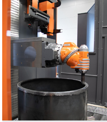
Turning operation for a "drum housing" on the milling center.
