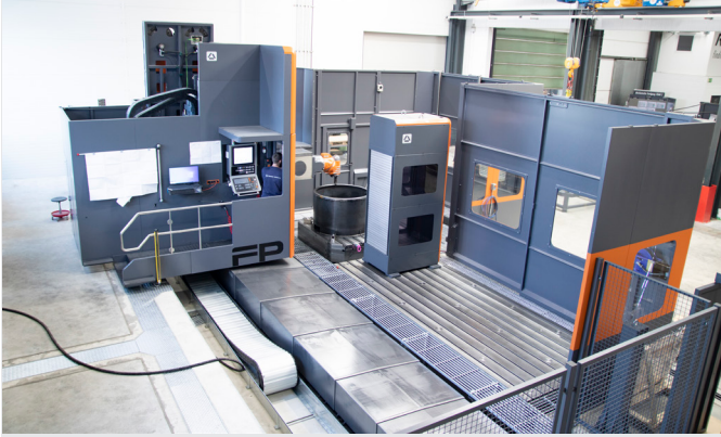
Full view of the moving column milling and drilling center.
