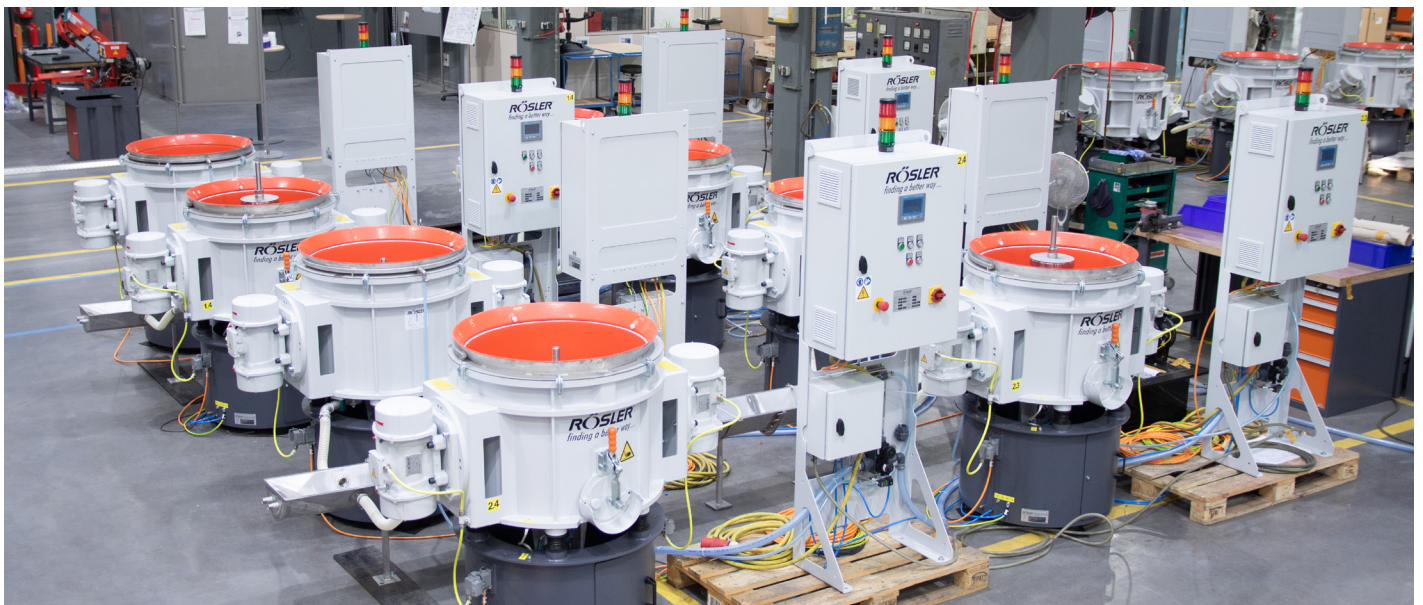
The pre-commissioning of the first 11 wheel finishing machines took place virtually in September 2021. With a live stream the 3-step mass finishing process in the FBA 24/2 was broadcast from Germany to the United States.
